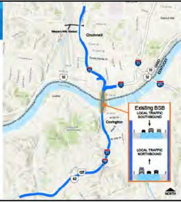
The existing double-decker Brent Spence bridge will be rehabilitated and reconfigured to reduce the number of lanes on each deck from four to three and provide inside and outside shoulders. The existing bridge will carry local traffic as part of the proposed collector-distributor roadway system.
