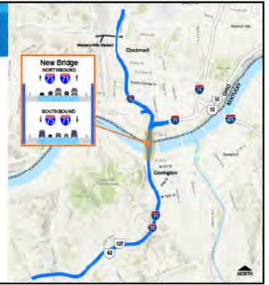
Between Ohio and Kentucky, the project will build a new double decker companion bridge with five lanes on each deck west of the existing BSB. The new bridge will carry through (interstate) traffic across the Ohio River.
