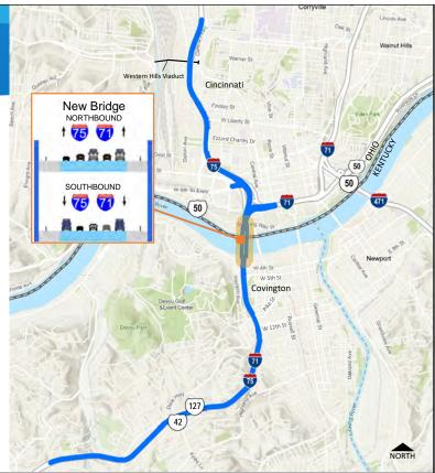
Between Ohio and Kentucky, the project will build a new double decker companion bridge with five lanes on each deck west of the existing BSB. The new bridge will carry through (interstate) traffic across the Ohio River.
