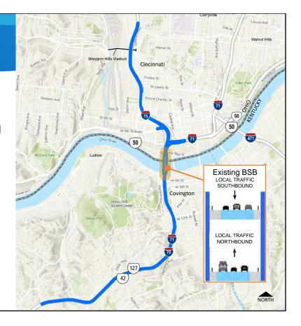
The existing double-decker Brent Spence bridge will be rehabilitated and reconfigured to reduce the number of lanes on each deck from four to three and provide inside and outside shoulders. The existing bridge will carry local traffic only as part of the proposed collector-distributor roadway system described earlier.
