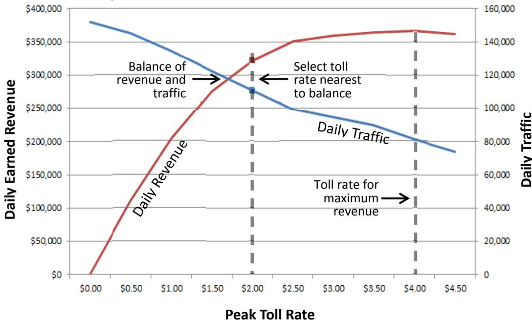
As an additional point for comparison, the toll rate that is forecasted to provide maximum revenue may be found using the same graph. Note that at the point at which the revenue is maximized, traffic using the toll road is much lower than at the point of balance. In the LSIORB example above, this toll rate is about \$4.
