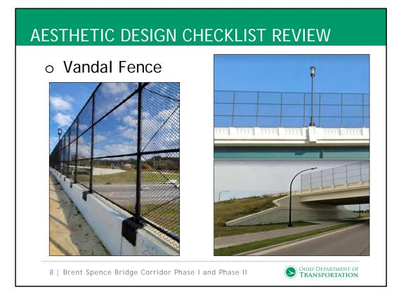
• The Vandal Fence proposed for the projects will consist of an ODOT standard Straight Black chain link Fence - 14' from the top of walk similar to what is pictured here and used in the corridor
