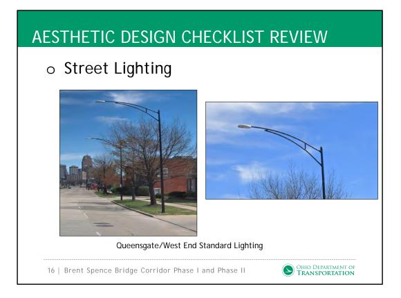
• Local street lighting will match the existing Queensgate/West End Standard which is a black Steel Tapered Pole with a Curved Truss Mast Arm
