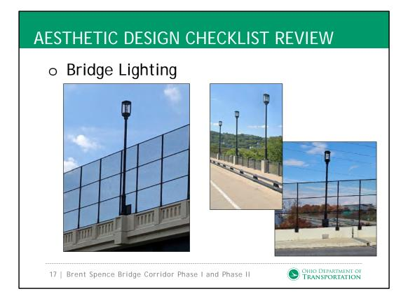
Overhead bridges will include a Straight Steel pole with Post top LED Luminaire matching the existing Hopple, Monmouth and West 8<sup>th</sup> Street bridges
